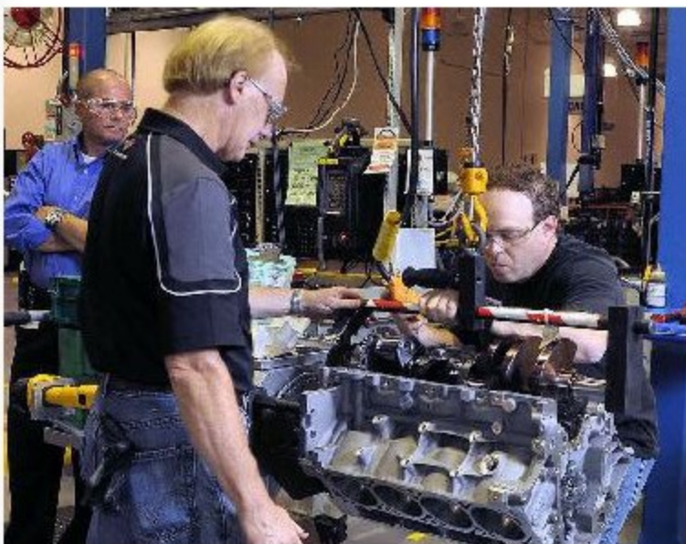
Todd Schnitt, above, places the crankshaft into the 638-horsepower supercharged small block engine for his 2011 Corvette ZR1 on Monday, August 30th, at GM's Performance Build Center with help from engine engineer Jordan Lebuilder, left, and engine builder Mike Priest.
