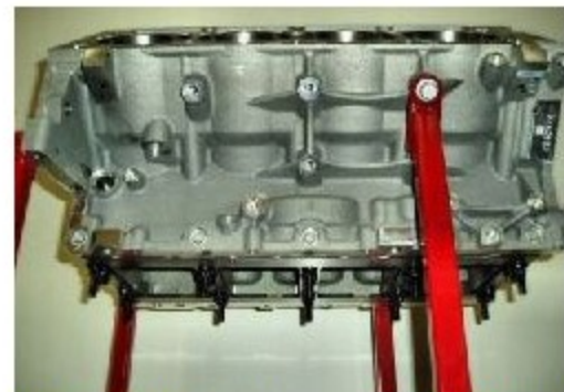
Picture #2 - Side view of C5R Block Note the water jacket does not extend beyond the piston movement area
